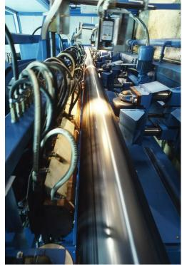
The steel pipes will be manufactured at Corinth Pipeworks' facilities and will include three-layer polyethylene external and epoxy internal coating, applied at the same location as the pipe manufacturing, at the Thisvi plant, in Greece.
